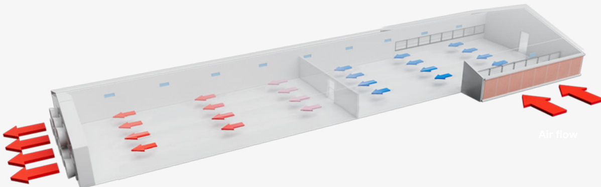
Figure 108 Air flow in a tunnel ventilated house.
